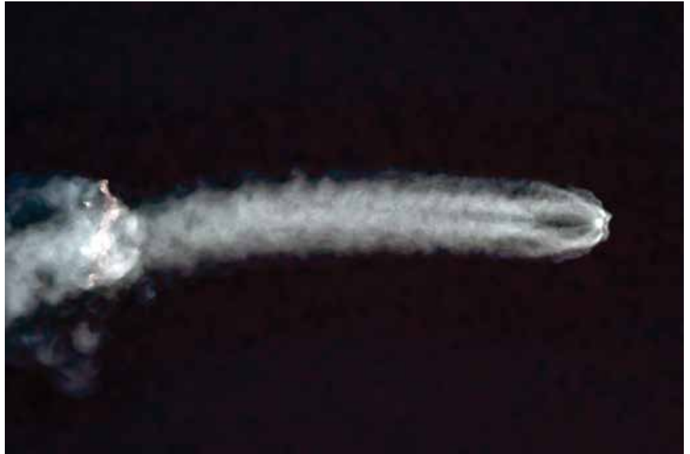
SpaceX Falcon heavy boosters separate from the center core and perform the boostback burn to return to Earth as the main rocket continues to space.
